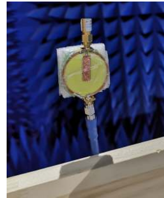
FIGURE 4. The antenna in microwave chamber for measurement.
