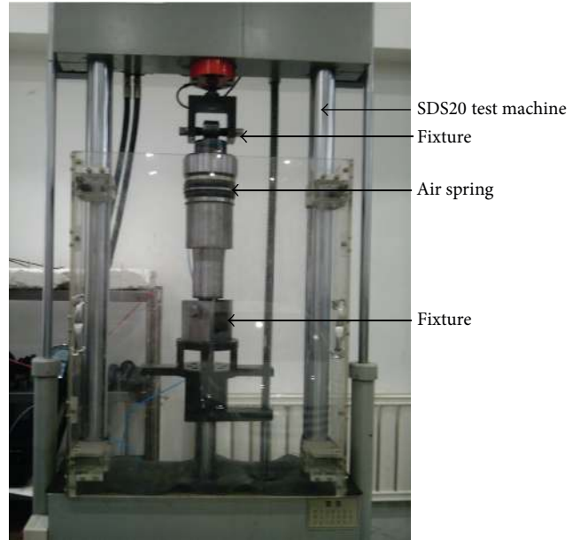
FIGURE 7: Static stiffness experiment of air spring.
