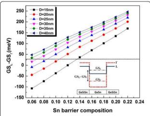
**Fig. 3** Directness parameter ( $GS_L$ - $GS_T$ ) variation as a function of the  $Ge_{0.72}Sn_{0.28}$  QD size and Sn composition of the  $Ge_{0.65-x}Si_{0.35}Sn_x$  surrounding layer. The dotted line indicates the thermal energy at room temperature. The inset represents a schematic definition of the directness parameter
