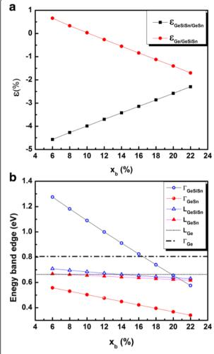
**Fig. 1 a** Lattice mismatch between  $Ge_{0.65 \times b}Si_{0.35}Sn_{xb}$  and Ge (filled circles) and between  $Ge_{0.72}Sn_{0.28}$  and  $Ge_{0.65 \times b}Si_{0.35}Sn_{xb}$  (filled squares) as a function of  $x_b$ . **b** Band edges at L and G valleys for  $Ge_{0.65 \times b}Si_{0.35}Sn_{xb}$ ,  $Ge_{0.72}Sn_{0.28}$ , and Ge as a function of  $x_b$
