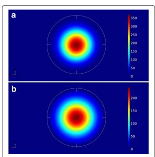
**Fig. 4** Squared electron ground state wave function for 35-nm-diameter  $Ge_{0.72}Sn_{0.28}$  QD for **a** Xb = 6% and **b** Xb = 22%
