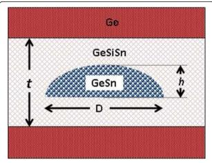
**Fig. 2** Schematic presentation of the modeled GeSn QD of height (*h*) and diameter (*D*) within GeSiSn strain-reducing layer in Ge matrix
