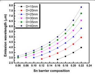
**Fig. 5** Room temperature ground state emission wavelength from direct bandgap  $Ge_{0.72}Sn_{0.28}$  QD as a function of size and Sn composition of the  $Ge_{0.65-xb}Si_{0.35}Sn_{xb}$  surrounding layer
