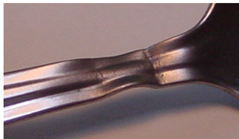
Figure 2.50 Close-up of bending area showing fatigue cracks appearing
