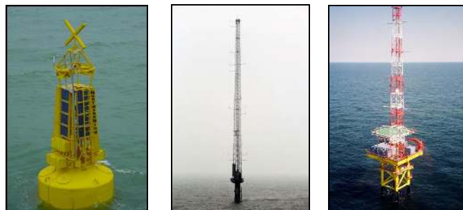
Figure 3.3 Wave and wind measurement buoy at OWEZ, met-mast at Horns Rev, FINO platform north of Borkum
