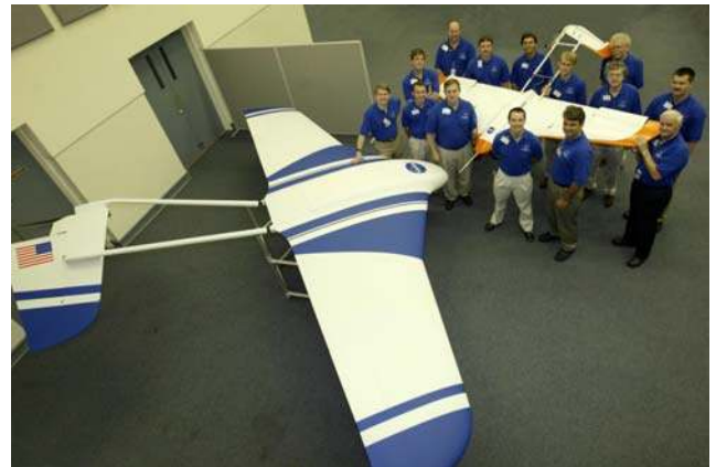
Figure 12: Mars airplane half- and full-scale flight test vehicles. The half-scale vehicle has relevant geometric, folding scheme and airfoil characteristics. In addition to aerodynamics, the full-scale vehicle was designed with a flight-like composite structure, capable of withstanding launch loads.
