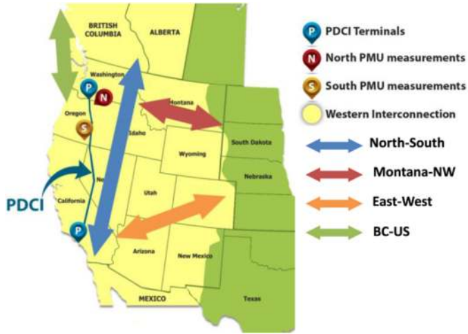
Fig. 1. Modes of oscillation in the North American Western Interconnection. The typical modal frequencies are: North-South B \sim 0.4 Hz, North-South A \sim 0.25 Hz, Montana-NW \sim 0.8 Hz, East-West \sim 0.5 Hz, and BC-US \sim 0.6 Hz.
