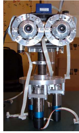
Fig. 4. Prototype of robot head with spring-based neck.
