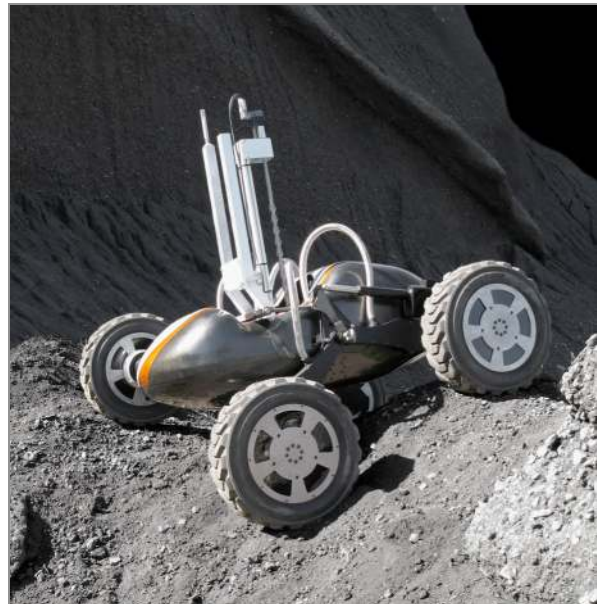
Figure 7: Suspension conforming to terrain
