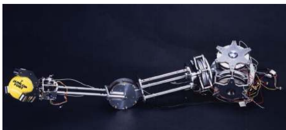
Fig. 4 An artificial arm by using the spherical ultrasonic motor
