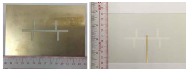
FIGURE 11. Photograph of the prototype antenna fed by a 50- \Omega short-ended microstrip line.
