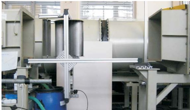
Installation of Savonius turbine at the test section
