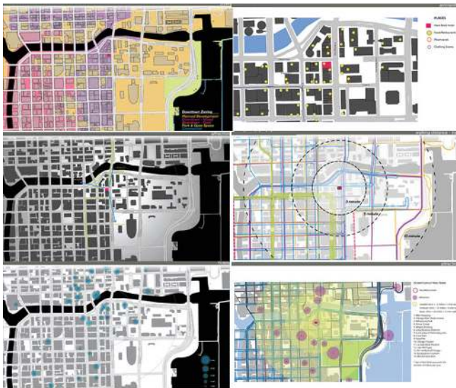
Figure 1. Site Analysis Diagrams: Views, Zoning, Transportation, Walkability, Demographics, Retail and Residential Programs around the site. This information is used to set up the parametric massing model on the site.
