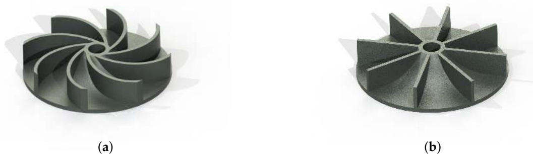
Figure 5. Schematic view of impellers (a) with curved blades; and (b) with straight blades.
