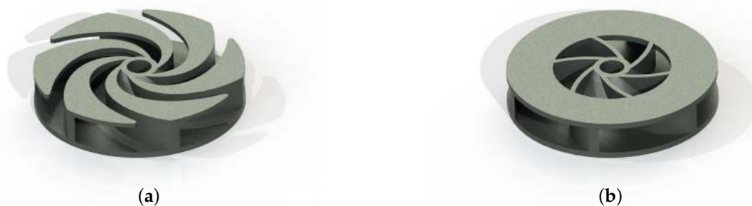
Figure 6. Schematic view of impellers (a) with winglets; and (b) with front shroud.
