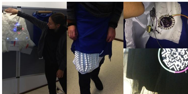
Figure 8. On the left, the skirt with a proximity sensor. Remaining images are of the skirt for dementia: comfort balls, the GPS and a QR code.
