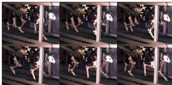
Fig. 12. High-speed video captured at 500 fps depicting 150 ms of the MIT Cheetah running at 6 m/s
