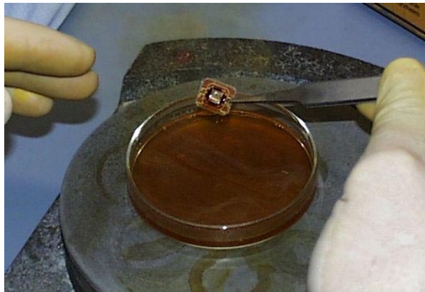
Figure 1: Hot fuming nitric acid ( > 98\% \text{HNO}_3 ) dissolves the package without affecting the chip.
