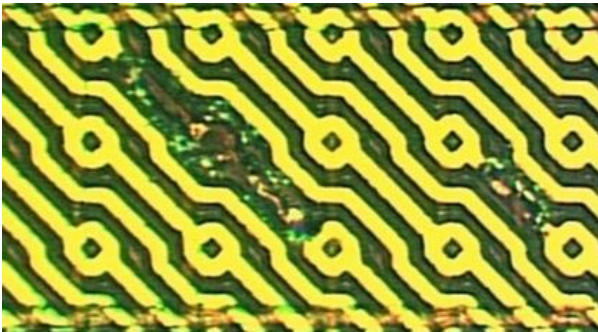
Figure 10: Every second line is connected to VCC or GND at one end and open at the other. Not all are used to supply lower layers and therefore some can safely be opened with a laser for probing access to the bus lines below.
