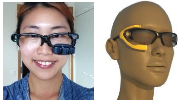
Figure 1. Smart glasses design probe in use by a test participant (image taken from participant's self-recorded diary), and example of the created industrial designs.
