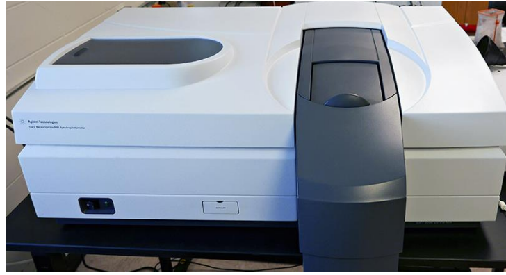
Figure 3.18 UV-Vis-NIR Agilent Cary 5000 spectrophotometer used at Polytechnic University of Turin.
