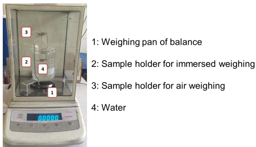
Figure 3.7 Density set-up used at Polytechnic University of Turin.
