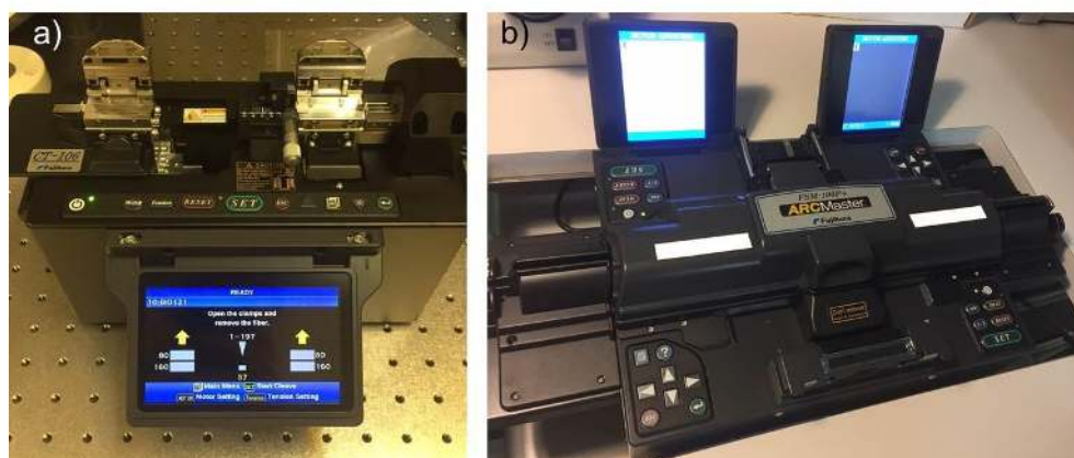
Figure 3.24 (a) Cleaver equipment (Fujikura CT-106) and (b) the splicer equipment (Fujikura FSM-100P+) used at Polytechnic University of Turin.
