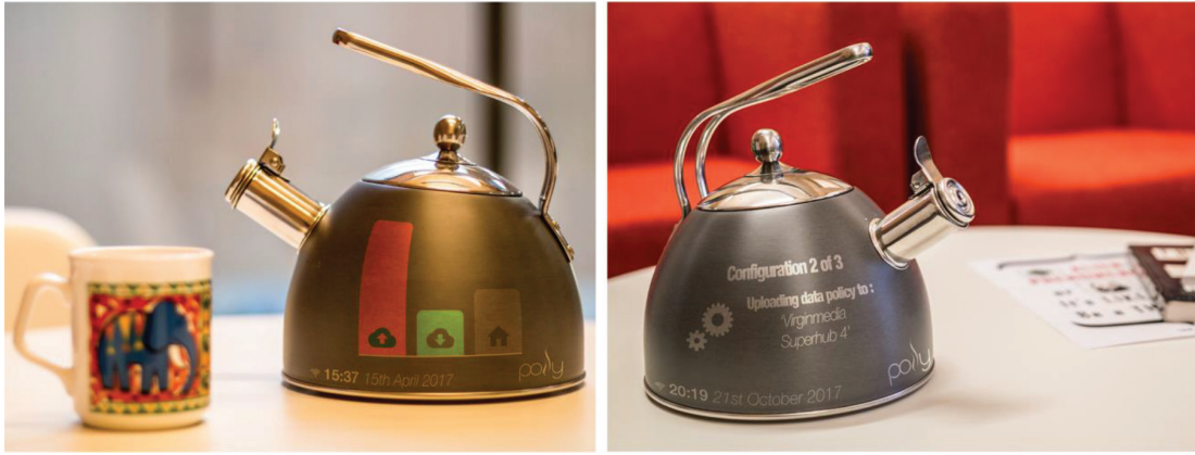
Figure 4: Features associated with the Polly kettle’s “OOO rhetoric”. On the left a visual display lets the user know the volume of data the kettle is downloading relative to uploads and local network traffic. On the right a machine reading data policy is uploaded from the kettle to a compatible router.
