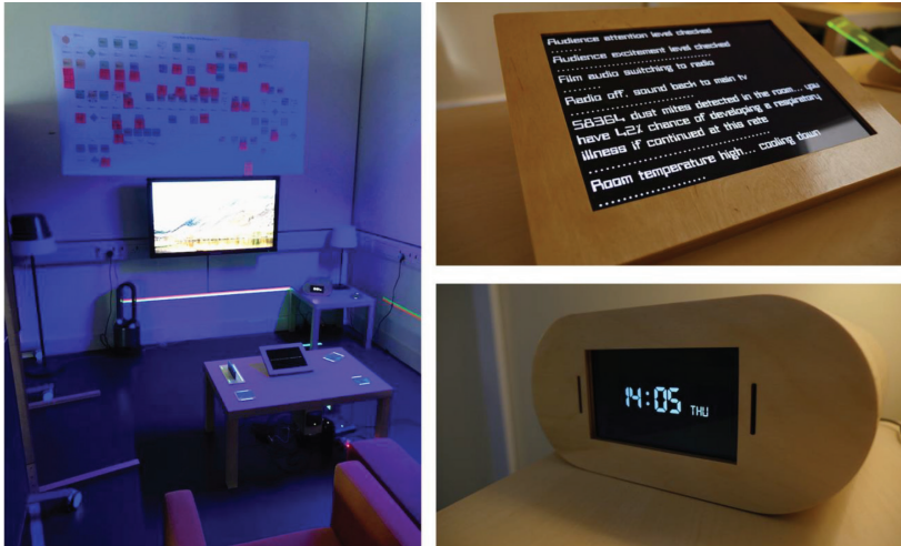
Figure 15: A UV light was used as an output object to highlight connections between other objects, as well as augmenting the media performance at key moments (left). Custom-made tablet (top right) and clock radio (bottom right) provided visual and audio augmentations.
