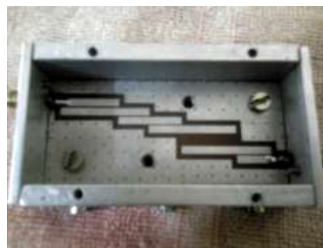
Fig. 8 Fabricated microstrip parallel coupled line band pass filter
