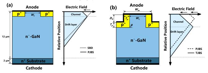
peak moves further into the drift layer due to the adoption of the trench and allows the formation of deeper pn junction.
