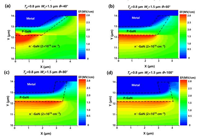
**Figure 8.** Local 2-D electric field distributions of TJBS diodes with a  $\theta$  of (**a**) 40°; (**b**) 60°; (**c**) 80°; and (**d**) 100° with a p-doping concentration of 2 × 10<sup>17</sup> cm<sup>-3</sup> at a reverse bias of 1000 V.
