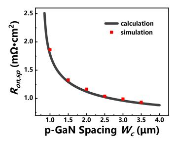
**Figure 10.** Comparison of the specific on-resistance calculated from the resistance analysis model with the simulation results for TJBS diodes with  $\theta = 60^{\circ}$ .
