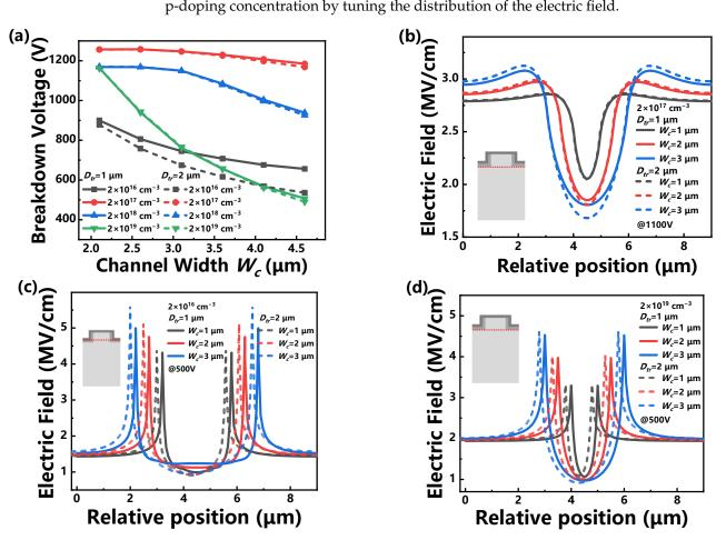
of the TJBS diodes, jointly determining the breakdown voltage of the devices with the p-doping concentration by tuning the distribution of the electric field.
