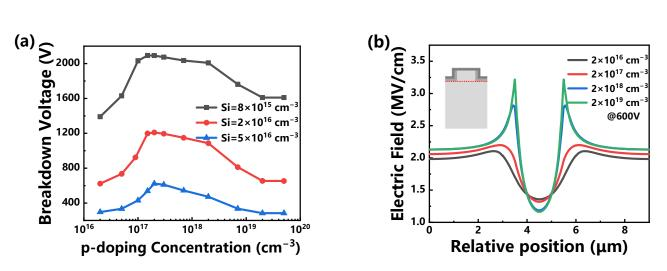
**Figure 3.** (a) Breakdown voltage as a function of p-doping concentration for TJBS diodes with different drift layer concentrations; and (b) electric field profiles along the bottom of p-GaN for TJBS diodes with different p-doping concentrations at the reverse bias of 600 V when the drift layer concentration is  $2 \times 10^{16}$  cm<sup>-3</sup>.
