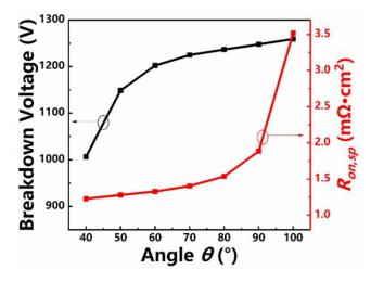
**Figure 7.** Breakdown voltage and on-resistance of the TJBS diodes as a function of the variation of the angle ( $\theta$ ) of the trench slope.
