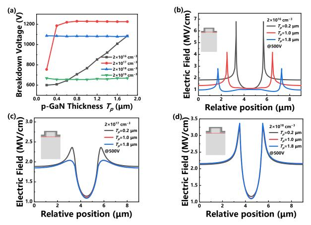
Figure 5. (a) Breakdown voltage of TJBS diodes with different p-doping concentrations as a function of
