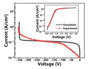
**Figure 2.** Forward bias (inset) and reverse breakdown comparison of the simulated and experimental data. Adapted from [29].
