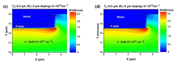
**Figure 4.** Local 2-D electric field distributions of TJBS diodes with p-doping concentrations of (**a**)  $2 \times 10^{16}$  cm<sup>-3</sup>; (**b**)  $2 \times 10^{17}$  cm<sup>-3</sup>; (**c**)  $2 \times 10^{18}$  cm<sup>-3</sup>; and (**d**)  $2 \times 10^{19}$  cm<sup>-3</sup> at 600 V reverse biased and a drift layer concentration of  $2 \times 10^{16}$  cm<sup>-3</sup>.
