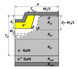
Figure 9. Current path in TJBS diode used for on-state analysis.
