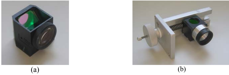
Figure 6. Detailed photographs of (a) a standard commercial cube for a Nikon Eclipse TE-2000E microscope and (b) a custom-made cube for a Motic AE-31 microscope.
