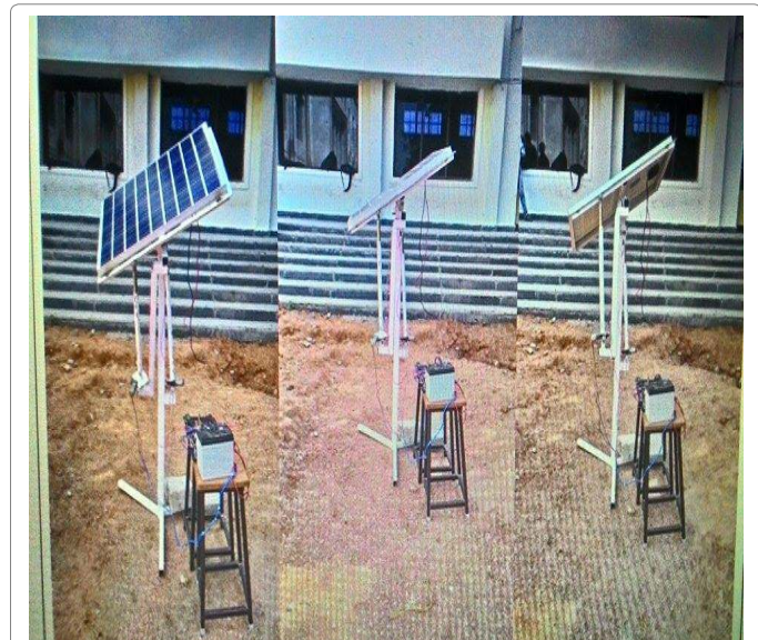
Figure 4: Solar tracking set up.
