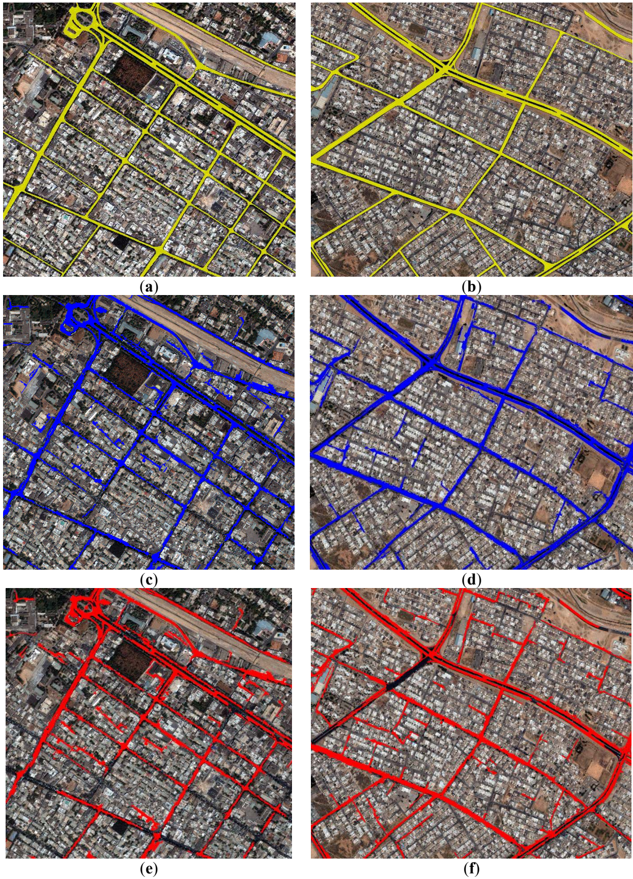
Figure 13. (a,b) The referenced road data of Hamadan 1,2 IKONOS images. (c,d) The final result of the proposed T2 FLS after enhancement. (e,f) The final result of T1 FLS after enhancement.
