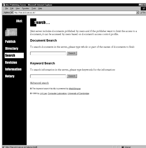
Figure C.4. Search menu: the screen shows the form used to search for published documents. Documents can be sought by name, or by keyword; an advanced search facility is also provided.
