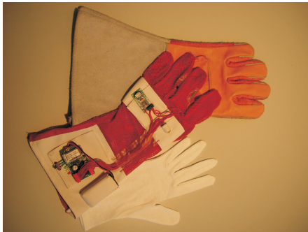
Fig. 1. Layer-based Wearing Concept of the Data-Glove
