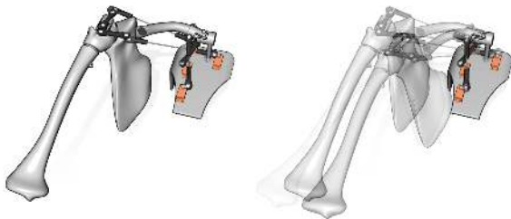
Fig. 13. The left image shows the shoulder mechanism and the right shows possible displacements.
