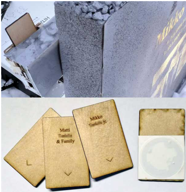
Figure 3: Closeup of the RFID tag reader integrated into the gravestone and examples of the wooden cards used to trigger display content
