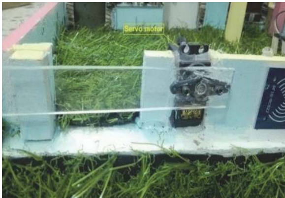
Figure 19. Design of the garage gate system
