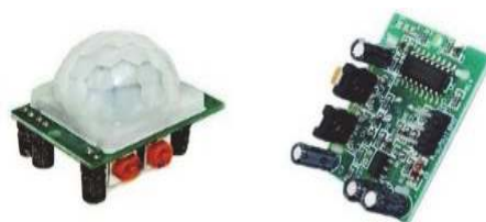
Figure 12. The PIR sensor
