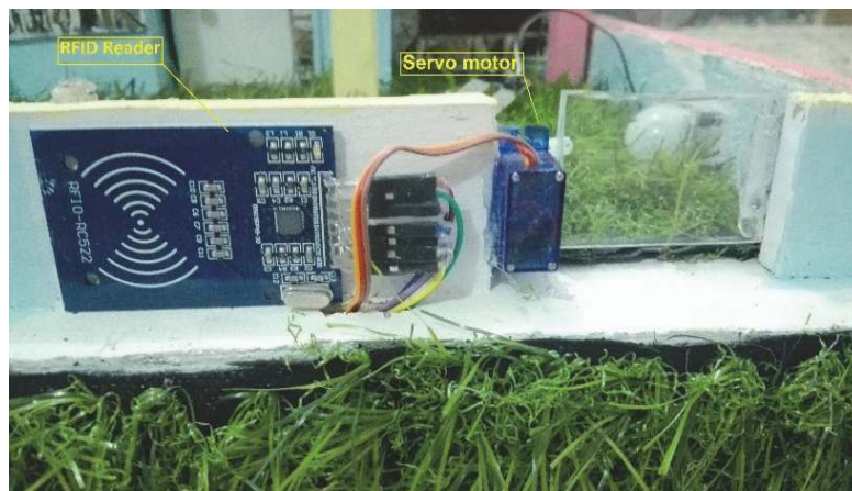
Figure 23. Implemented circuit of house main door with RFID
