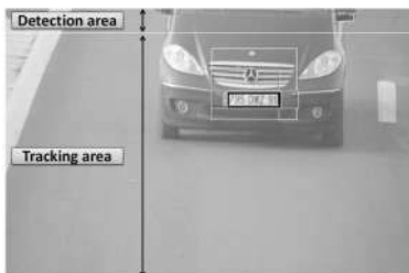
Figure 13: Number plate detection example
