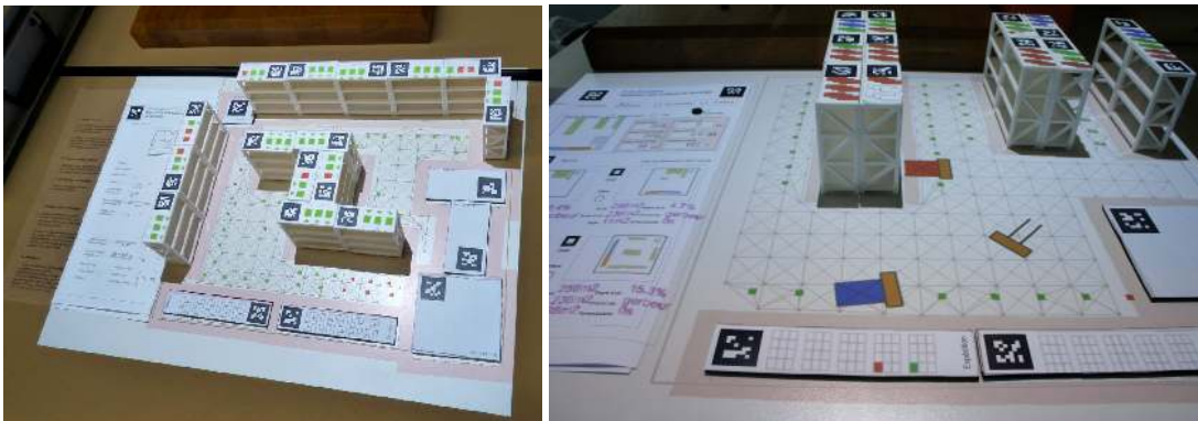
Figure 3. Shelf and navigation node augmentation on top of the small-scale model: a red square indicates that a pallet cannot be accessed by a forklift due to the lack of space (left). Simulation of a warehouse model: three forklifts are working in the warehouse (right).
