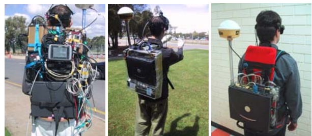
Figure 1 - The evolution of our Tinmith backpack designs (1) Unorganised design from 2001 with straps on hiking frame (2) Tinmith-Endeavour from 2002 with polycarbonate casing (3) New Tinmith backpack 2004 with compact box and frame
