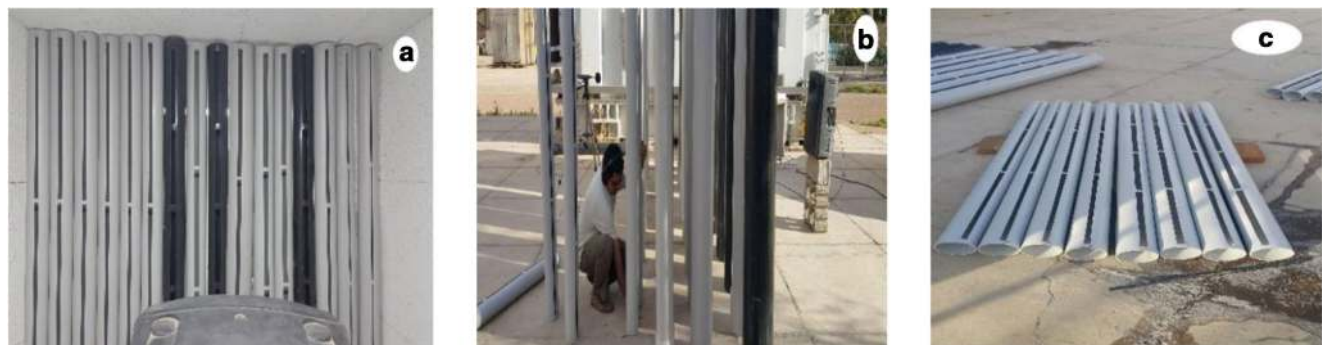
Fig. 15 a Frequency analysis and sound pressure level of pipes with 125 mm diameter inside the acoustic room b ) Symmetric and Non- symmetric array of pipe in free space c ) prepared pipe with slit before the tests
