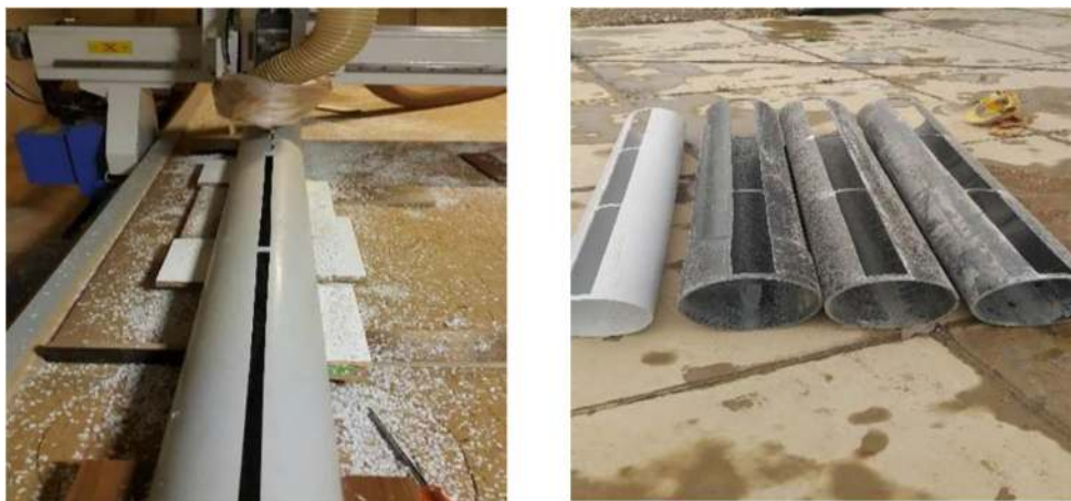
Fig. 11 Workshop area shows how to create CNC and necessary gaps in different size pipes to make IQFSCAB structures
