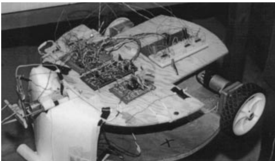
Fig. 1. The vehicle used for the contest with a controller mounted on top. The vehicle is equipped with optical triggering to start each heat, the drive motors and the batteries.
