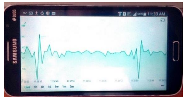
Fig. 8. ECG Output Signal on Blynk Application.
