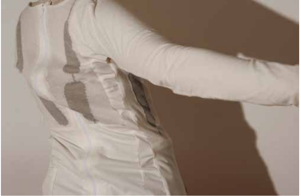
Figure 5.3: Picture of Vigour v1 (P14) with sensor areas on specific parts of the body that can be used to measure movement of the arms and lower back.
