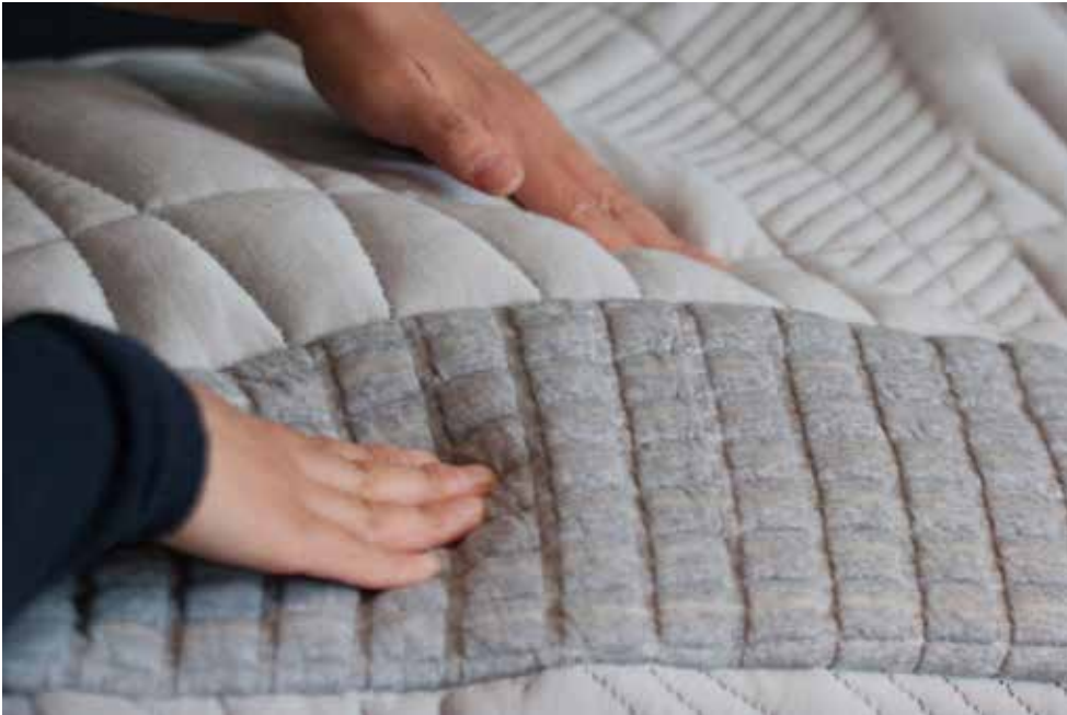
Figure 3.23: Tactile Dialogues v1 (P23) during an interaction session. The squares within the fabric contain the 3D-printed casings and the vibration motors. In the squared fabric itself, the touch sensors are also knitted into the fabric.
