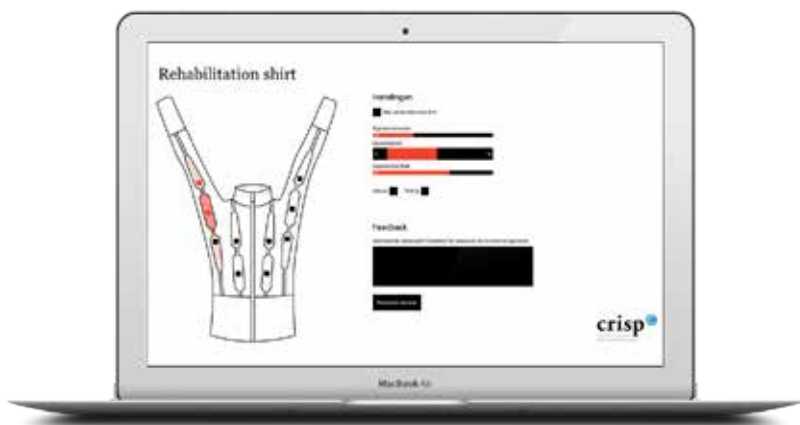
Figure 5.4: The interactive application Vigour v1 Interface (P13), that the therapist saw on the computer. The red parts on the shirt indicate which sensors are currently being stretched. With the bars on the right side, the therapists could change the sensitivity of the sensors.
