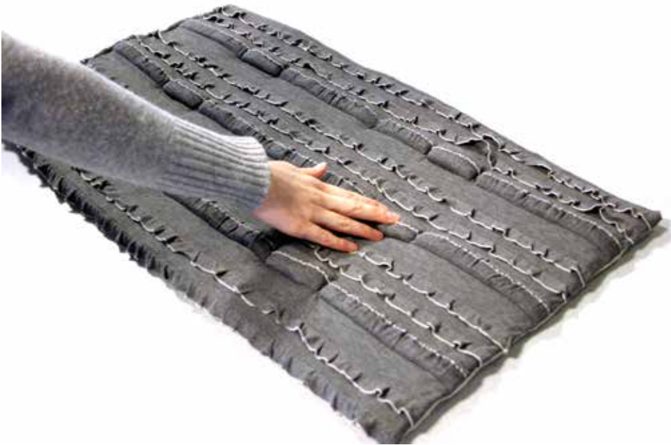
Figure 3.20: Blanket (P15) prototype. The bulky pockets (touched by the hand) contain the different actuators, such as vibration, light and sound. The seam on top of the pocket is sewn with conductive yarn, and is able to measure touch through capacitance.
