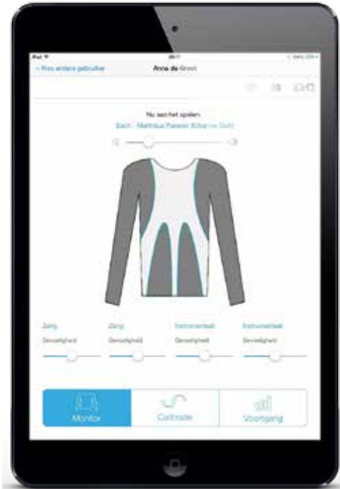
Figure 5.8: Interface for iPad (P21) that was developed by the Interaction Designer (S31), this screen shows the overview of the four sensors, and the instruments that can be connected.
