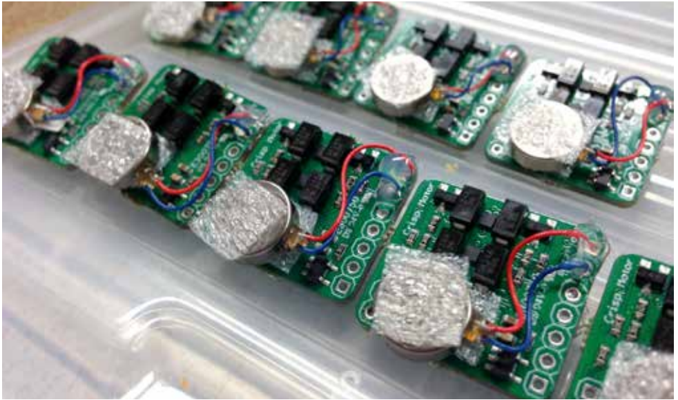
Figure 3.12: Some of the CRISP modules v2 (P17) with vibration motors added for integration in Vibe-ing.
