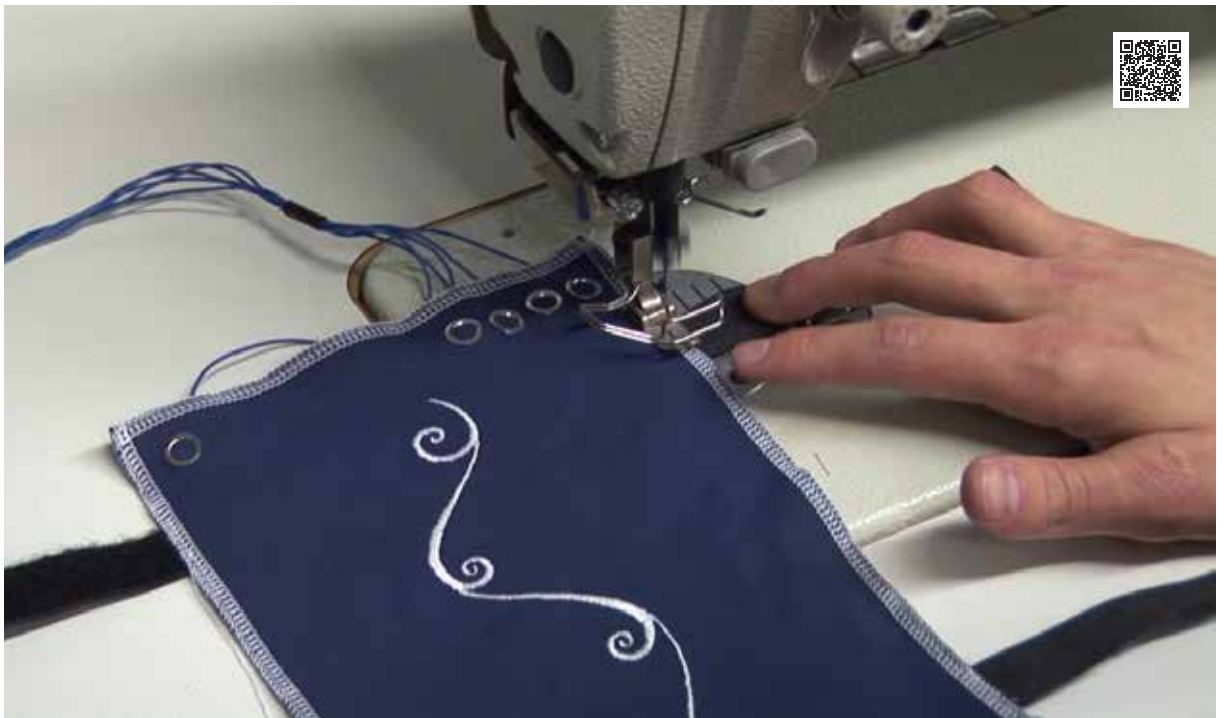
Figure 3.5: Constructing Music Fabric (P2) using techniques such as thermal bonding, embroidery, applying snaps, stitch-locking and sewing.
