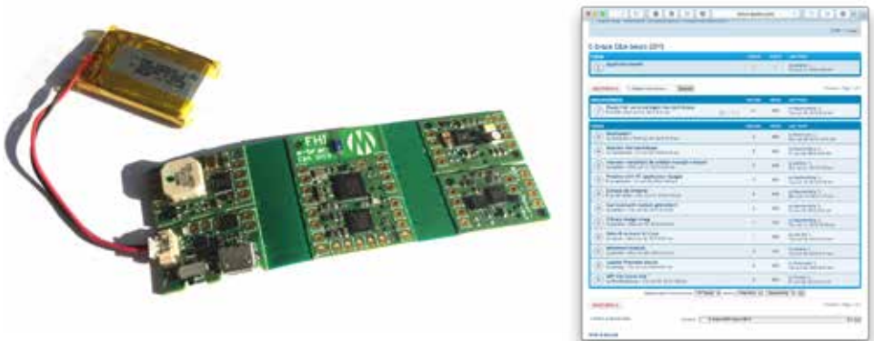
Figure 3.13: The new version of the CRISP modules, based on a flexible PCB connecting the modules, right: screenshot of the community forum where the software was open sourced.
