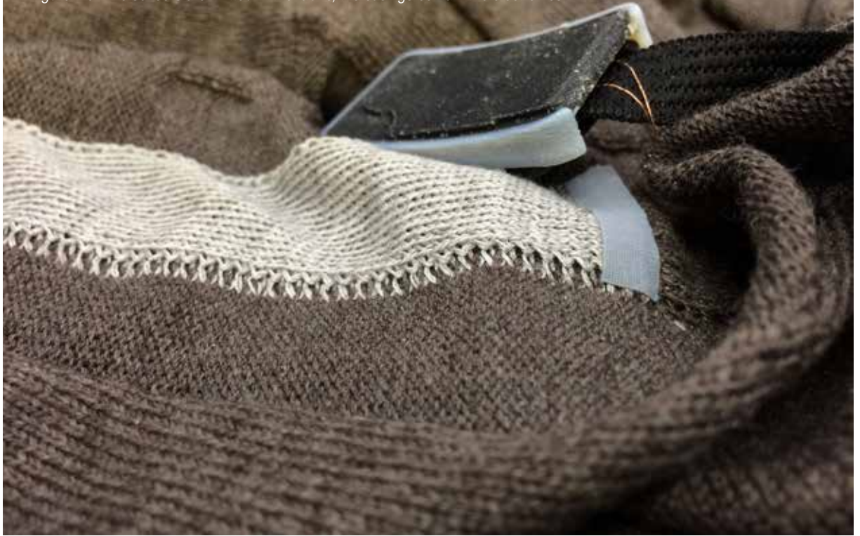
Figure 2.9: The sensors are knitted in the fabric, the casings contain the electronics.
