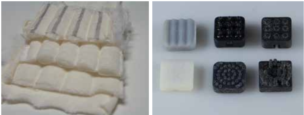
Figure 3.24: Left, several test pieces of fabric that have been knitted in the process to come to the final fabric. Right, exploration of several casings to contain the vibration motors within the fabric. The different surfaces on top aimed to explore different tactile sensations.
