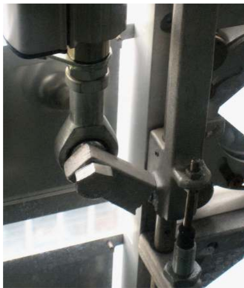
Figure 3 Mechanical diaphragms - image showing damage to the arm that transmits the force of the motor to the diaphragm actuation mechanism. Image: Author.
