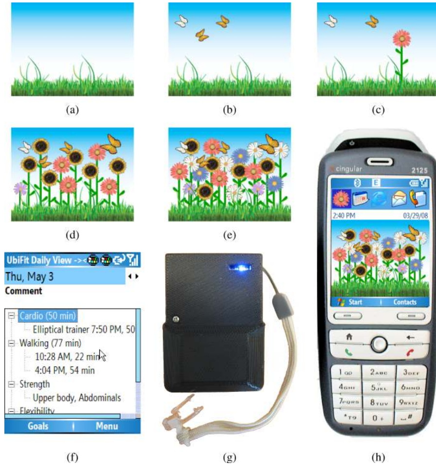
Fig. 1.2 An overview of UbiFit (a)–(e) show the glanceable display’s garden. In (a), the user has not performed any activities yet this week, and she did not meet her goal in any of the prior three weeks. In (b), the user has not performed any activities yet this week, but the three small butterflies indicate that she met her goal in each of the three prior weeks (yellow = primary goal, white = backup goal). In (c), the user has performed one cardio activity so far this week and met her goal last week and three weeks ago. In (d), the user has had an active week, but only performed cardio and walking activities. In (e), the user has had an active week full of variety. In (f), the user is looking at a daily view within the interactive application where her activities are broken down by category. In (g), the fitness device — i.e., the MSP — is shown, and (h) shows the garden as seen on the background screen of a Cingular 2125 Windows Mobile Smartphone.
