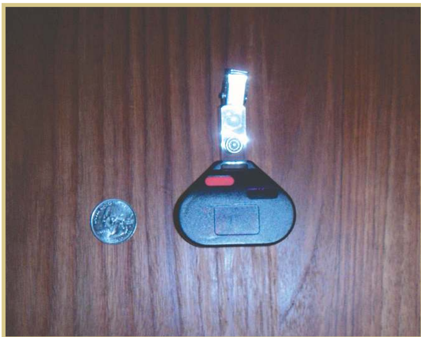
Figure 2. A mobile badge that broadcasts identification in infrared for indoor location monitoring and in radio frequency for outdoor, on campus location monitoring.
