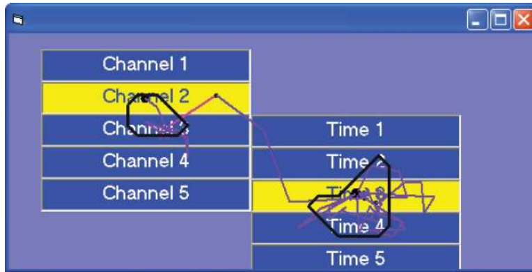
FIG. 26. Possible cursor trace of a pointing device (like mouse) operated by a person having motor impairment (color figure available online).
