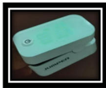
Fig. 11. Oximetry BLE Pulse Sensor Testing.
