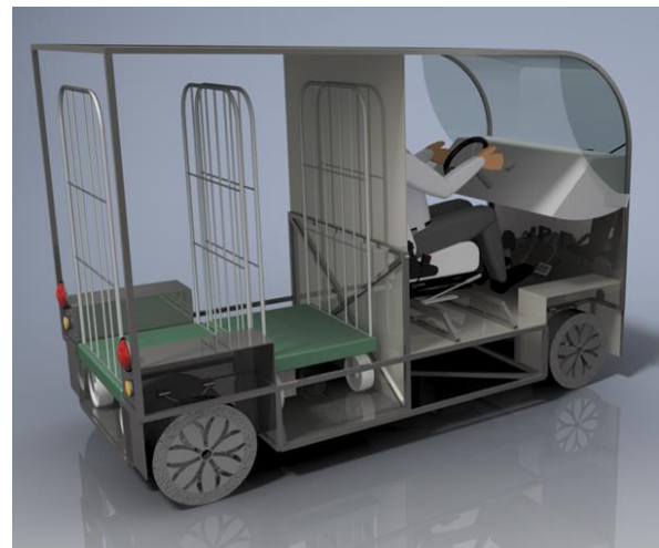
Figure 5: The vehicle design with two rolling containers
