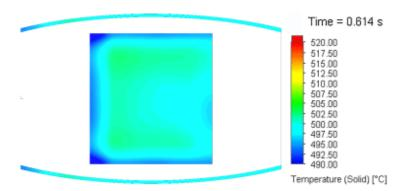
Figure 30. Temperature distribution over the plate (blade) surface at 0.614 s
