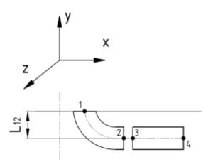
Figure 17. A scheme of the Euler turbine modification (a version, when  $R_1 < R_2 < R_3 < R_4$ ;  $\alpha_2 = \alpha_3 = 90^\circ$ )
