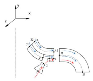
Figure 23. A scheme of a mesh turbomachine (option with two rows of blades), developed using the basic scheme of the Euler turbine
