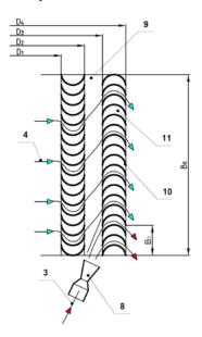
Figure 4. Schematic development drawing of the impeller blade system, according to application 2022110755
