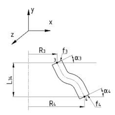
Figure 15. A scheme of the rotor for the Euler turbine (basic version)
