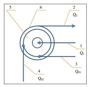
Figure 10. A turbomachine scheme (option 1): 1 – inlet channel for the pumped medium; 2 – outlet channel for a mixture of the working and the pumped media; 3, 4 – input channels for the working medium; 5 – rotor; 6 – body
