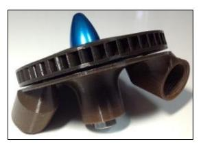
Figure 6. A photo of the created prototype – an impeller with a nozzle assembly (prototype version), according to application 2022110755
