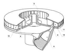
Figure 5. Impeller with nozzle assembly (3D model – isometric projection), according to application 2022110755
