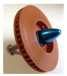
Figure 21. An impeller for a hybrid mesh turbomachine (prototype version according to application 2022110755): a photo of the micromodel – a view from the pumped medium inlet side
