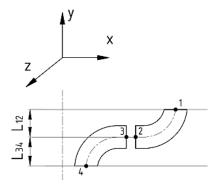
Figure 18. A scheme of the Euler turbine modification (a version, when  $R_1 > R_2 > R_3 > R_4$ ;  $\alpha_2 = \alpha_3 = -90^\circ$ )
