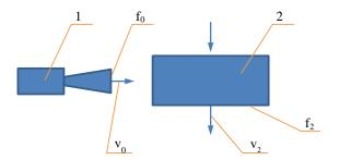
Figure 8. Scheme of the jet system for the energy converter: 1 – the working medium source; 2 – the working chamber
