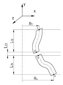
Figure 13. A scheme of the Euler turbine (basic version)
