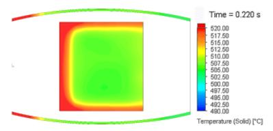
Figure 29. Temperature distribution over the plate (blade) surface at 0.220 s
