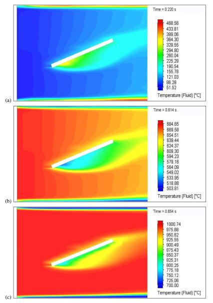
Figure 31. Distribution of gas temperature for different moments of time: a) 0.220 s; b) 0.614 s; c) 0.654 s
