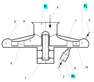
Figure 2. Scheme of the developed and patented turbomachine, according to application 2022110755: 1 - body;  $2 - outlet channel (pressure <math>P_2$ );  $3 - inlet channel for the working medium (pressure <math>P_0$ );  $4 - inlet channel for the pumped medium (pressure <math>P_1$ ); 5 - mixing chamber; 6 - impeller; 7 - shaft; 8 - nozzle apparatus; 9 - annular channel; 10 - turbine blades.
