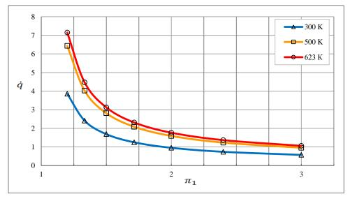
Figure 12. The calculated dependences of q' on π\_1at different working gas temperatures: 300 K (calculation-1); 500 K (calculation-2); 623 K (calculation-3)
