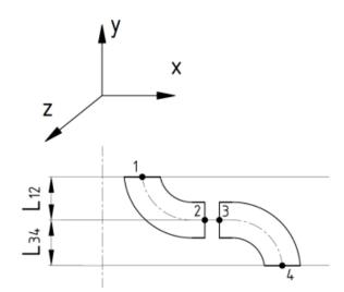
Figure 16. A scheme of the Euler turbine modification (version, when  $R_1 < R_2 < R_3 < R_4$ )
