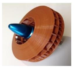
Figure 24. An impeller for a hybrid mesh turbomachine (prototype version with two rows of blades): a photo of the micromodel – a view from the side of the pumped medium inlet
