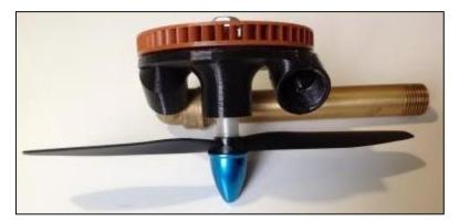
Figure 9. A photo of a jet system micromodel for energy conversion: a turbofan with a pusher propeller placed at the bottom (prototype version)
