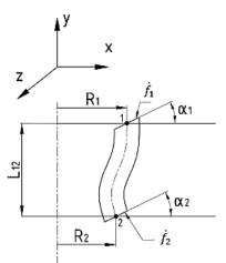
Figure 14. A scheme of the guide vane channel for the Euler turbine (basic version)
