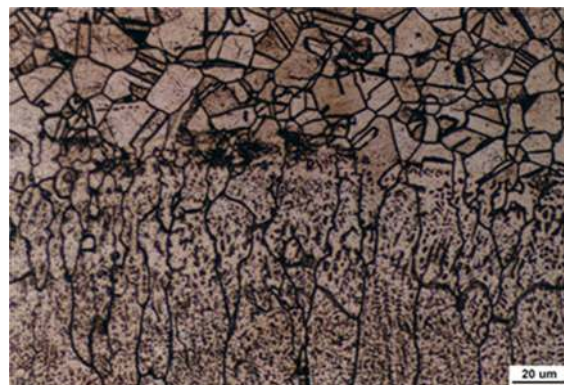
Figure 11. Connected network of carbides in type-B specimen PWHTed at 700 °C for 10 hours.
