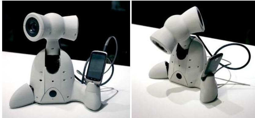
Figure 17. Completed prototype of Travis, a robotic speaker dock and listening companion.
