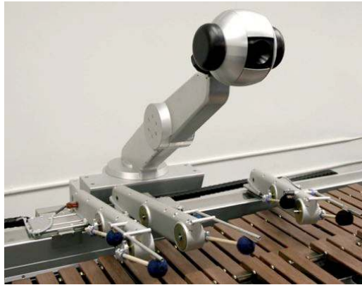
Figure 10. The socially expressive head of the robot “Shimon,” fully assembled and installed by the marimba-playing arms.
