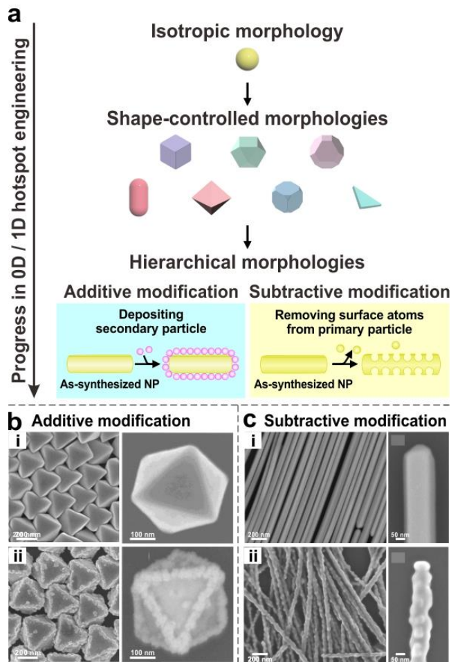
Figure 2. Emerging strategies for 0D/1D hotspot engineering. (a) Overview of the progress in 0D/1D hotspot engineering. (b) Additive post-synthetic modification. (i, ii) SEM images of as-synthesized Ag octahedron and selective edge Au-deposited Ag octahedral (SEGSO), respectively. (c) Subtractive post-synthetic modification. (i, ii) SEM images of as-synthesized Ag nanowires and etched Ag nanowires, respectively. Reprinted and adapted with permission from (b) ref 25 and (c) ref 23. Copyright 2014 John Wiley & Sons, Ltd. Copyright 2012 American Chemical Society.
