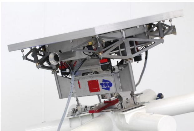
Figure 1: The 2010 prototype for the M1 segment support structure.
