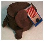
**Dream-Bot**. This robot-dog has the particularity of using a LED display to generate five different faces according to the situation. It can also be guided using a leash attached to a joystick located on the back of the robot.
