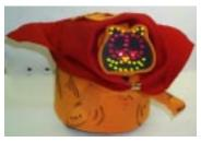
**SuperG**. This Garfield robot can talk and sing. Its special face built using LEDs is mounted on a servo-motor, along with its moving tail. Both are used to express the mood of the robot. Contact switches are used to pet the robot. When happy, SuperG also starts to purr. A keyboard placed under the cape is used to select different behavioral configurations. By clapping, the robot could also be directed to move or to stop.
