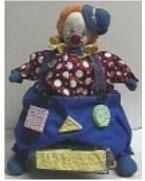
**CARI**. This robot-clown asks the child to play to three different games: to dance, to press on the round, the triangular or the square shape push buttons, or to pursue the robot. The head of the robot is mounted on a servo-motor and eyes are made with green LEDs. The legs of the robot are attached to the wheels to go up and down when the robot moves.
