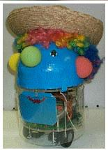
M³. This clown is programmed to call the name of the child as it moves. It can dance and play with the child using its nose and ears to interact. It smiles or shows signs of sadness depending on the situations. At the end the robot can give some candy to the child by opening its mouth, made using a CD-ROM reader.
