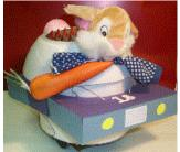
**FLIP**. This robot is designed to portray a rabbit in a car. It has a LED panel on its back to communicate different things to the child. The robot also has a memory game, music and can be tickled.
