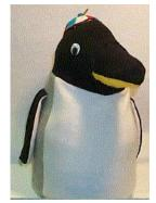
**TOBY**. This penguin can follow a light source and when it detects a loud noise, the propeller on top of its hat starts to turn. Clapping is used to start the robot. The robot also comes equipped with a console used in a game where the robot asks the child to correctly identify an object. Students in this team also found a way to improve the sound generation device.
