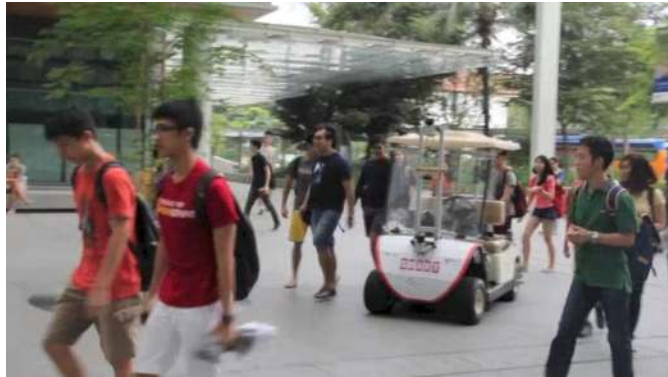
Figure 2: DESPOT running in real time on an autonomous golf-cart among many pedestrians.
