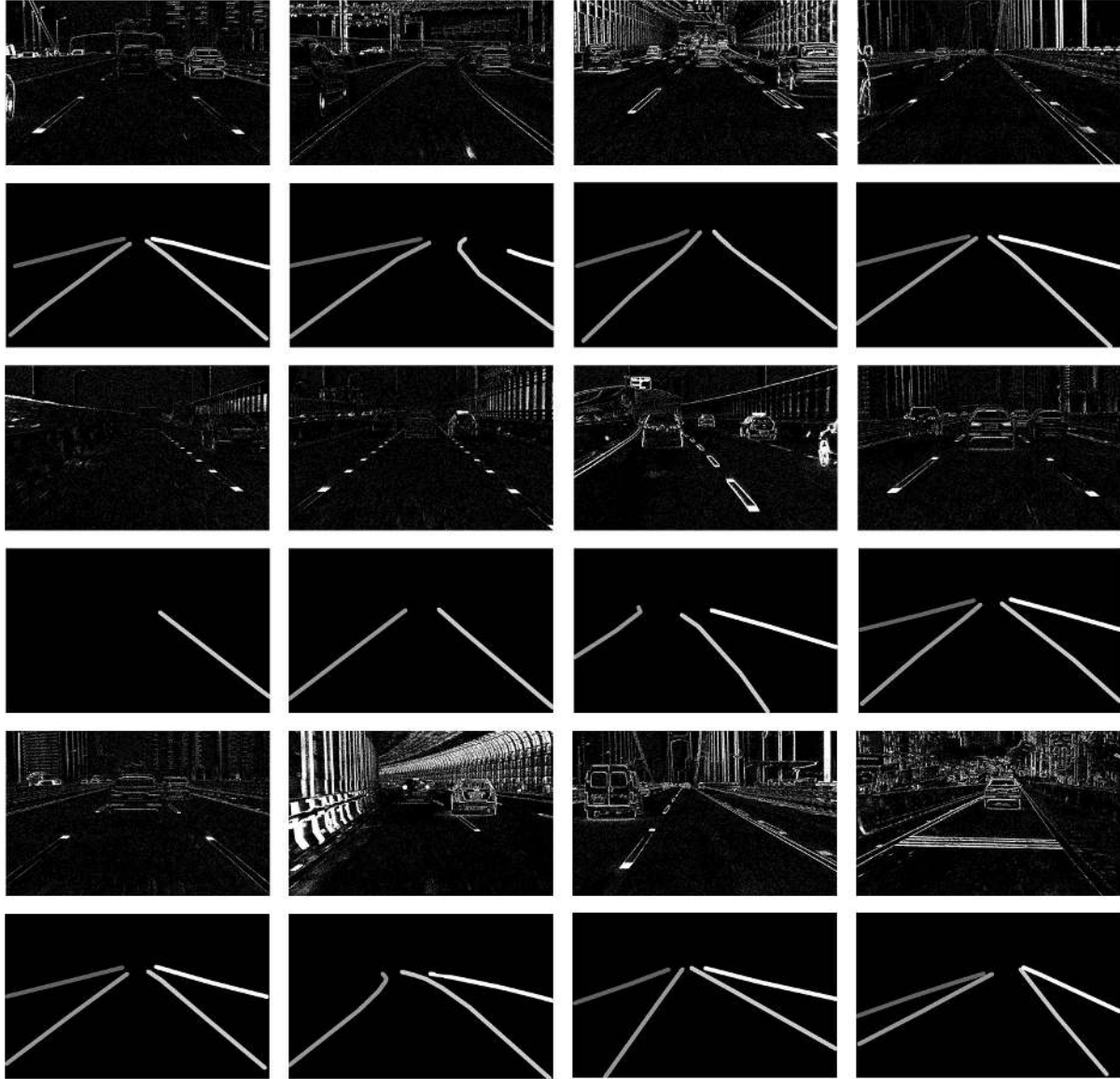
Figure 5. Samples of DVS images and labels in DET. First rows show various line types, including single dotted line, single solid line, parallel dotted line, parallel solid line and dotted line. Middle rows show various lane number, from 1 to 4. Last rows show various traffic scenes, urban, tunnel, bridge and overpass.
